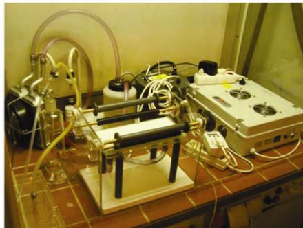
Figure 9. DBD laboratory test equipment used for polymer surfaces. [19]
