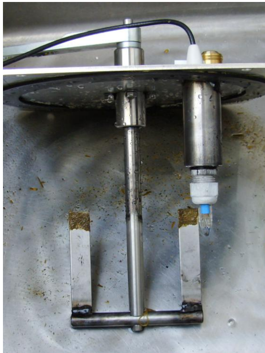
Fig. 4. Tested mixing paddle for homogenization
