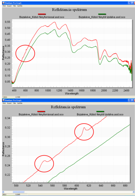
Fig. 7. Spectral disturbance caused by unfavored light infiltration
