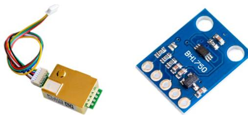
Figure 5. CO<sub>2</sub> content sensor and lighting sensor
