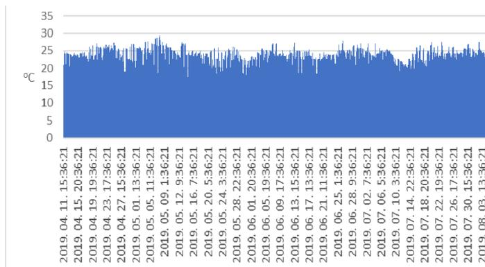
Figure 4. Measured internal temperature in an accommodation container
