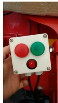
Figure 6. Control panel of INO Smart Hopper (Source: INO)
