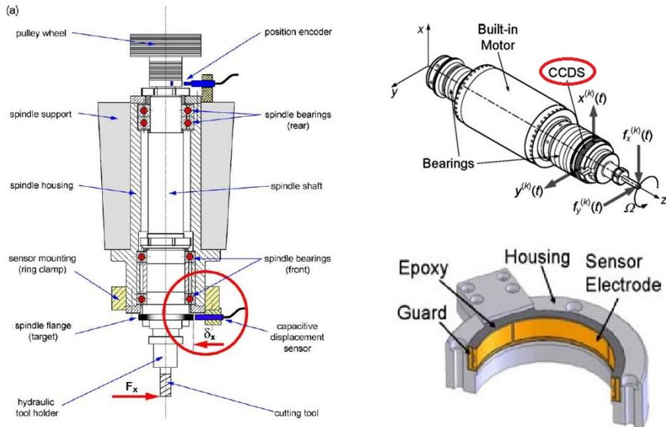
Figure 7. Force measuring with capacitive displacement sensors [Albrecht *et al* 2004, Kim *et al* 2005]
