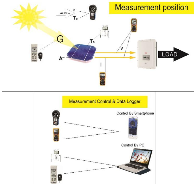
Figure 3. Data acquisition schematic diagram
