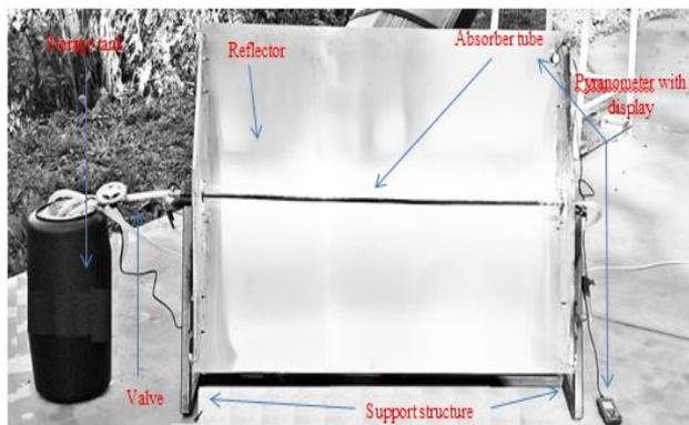
Figure 4. Components of PTSC System.
