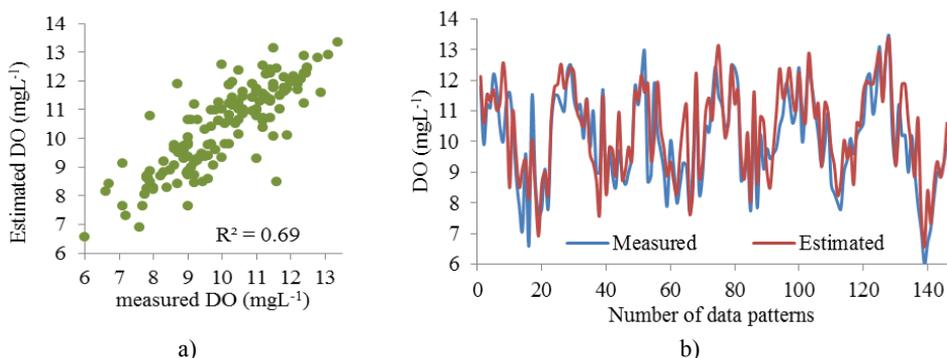
Figure 2. Scatterplot (a) and line chart (b) diagrams of measured and estimated DO at D<sub>A</sub>
