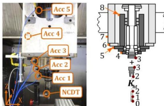
7. Figure Force measuring with accelerometers [Postel *et al* 2019]
