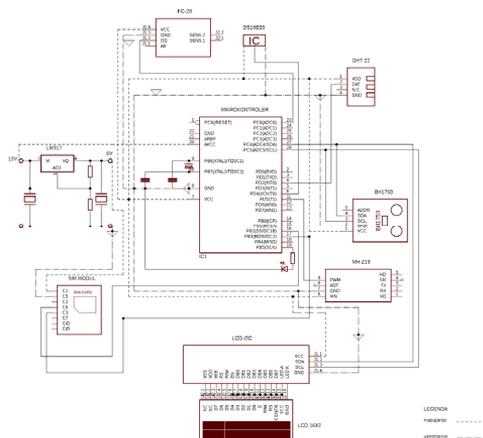
Figure 7. Electrical scheme of the device
