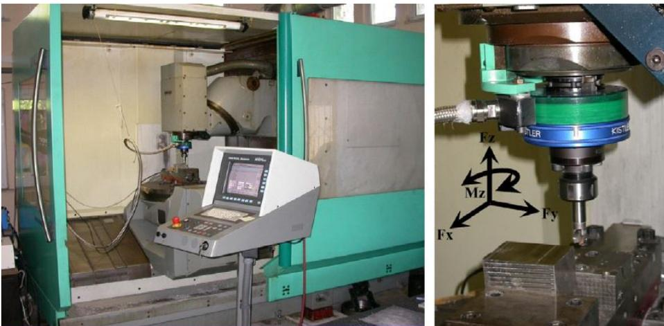
Figure 9. Experimental setup using a rotation force dynamometer [Kaya *et al* 2011]
