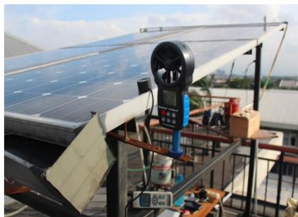
Data acquisition system for measuring  $G$ ,  $T_a$  and  $v$
