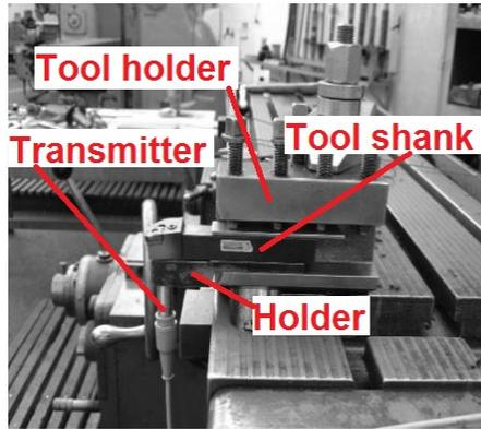
Figure 2. Force measuring with inductive transmitter [Kári-Horváth 2009]
