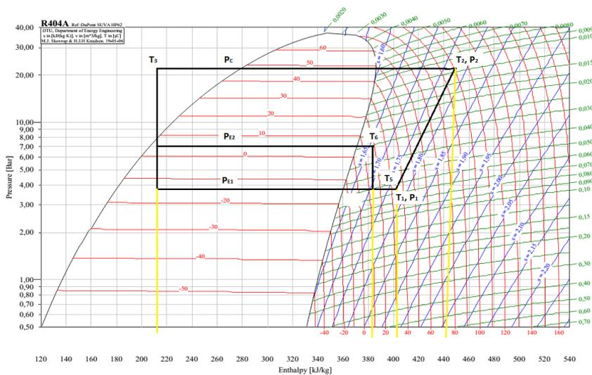
Figure 3. The cycle and the measuring points in logP-h diagram
