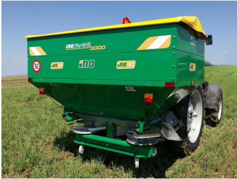
Figure 1. Double-disc mounted fertiliser spreader FERTI-2 (Source: INO)
