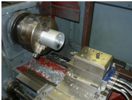
Figure 4. Kistler dynamometer for cutting force measuring
