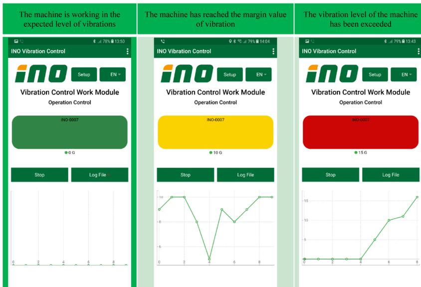
Figure 4. Three level of vibrations, normal, marginal, and excessive, showing on the mobile phone (Source: INO)
