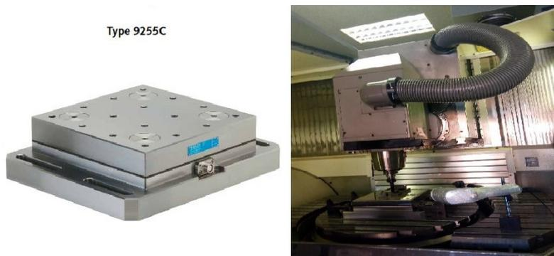
Figure 10. Force measuring with multicomponent dynamometer [kistler.com, Phokobye *et al* 2019]
