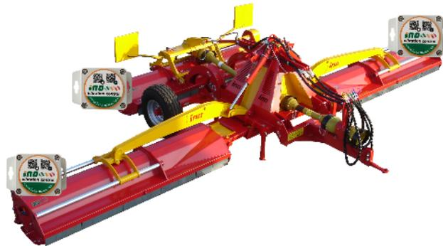
Figure 3. The position of the vibration sensors on the working machines, actually on the flail mower machine (Source: INO)
