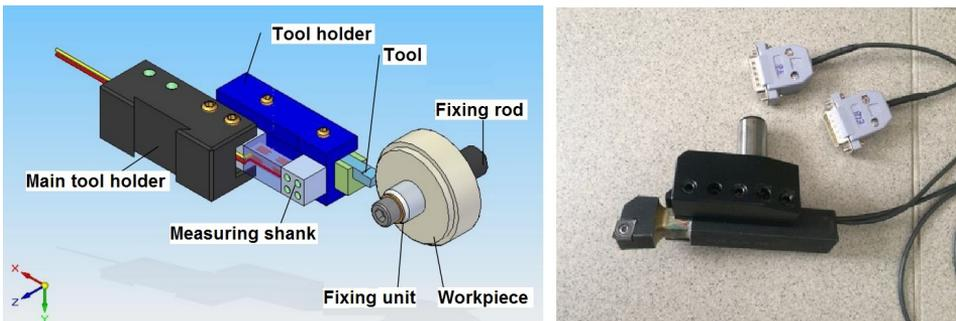
Figure 3. Force measuring units with strain gauges (Designed and created by Róbert Keresztes) [Dobrocsi 2011, Kovács 2016]
