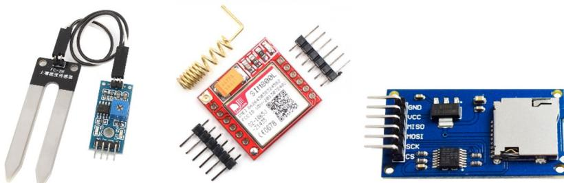
Figure 6. Soil moisture sensor, sim module and sd module
