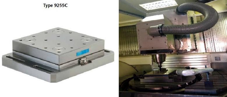
Figure 10. Force measuring with multicomponent dynamometer [kistler.com, Phokobye *et al* 2019]
