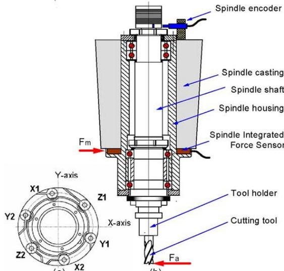
Figure 8. Force measuring method with combined sensors [Altintas *et al* 2004]
