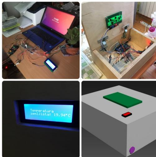
*Figure 8. Layout of prototype microclimate monitoring device*
