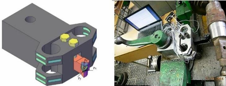
Figure 5. Special force measuring unit [Zablotskyi et al 2017]
