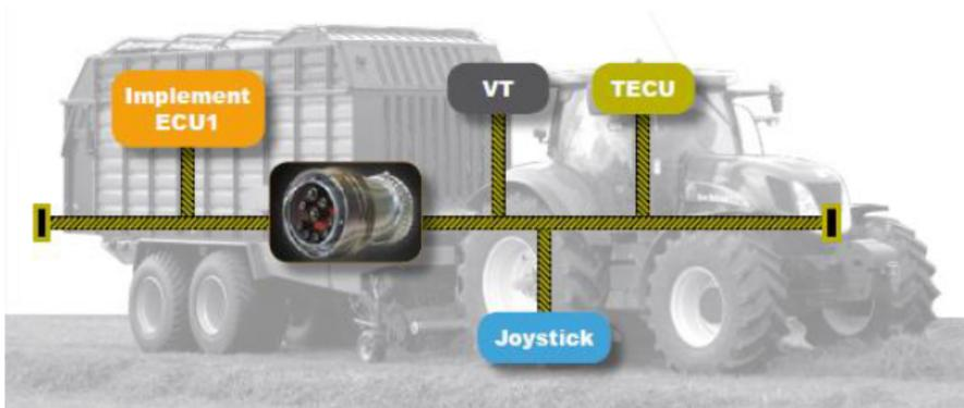
Figure 1. Typical standard ISOBUS System (Vlugt 2017)
