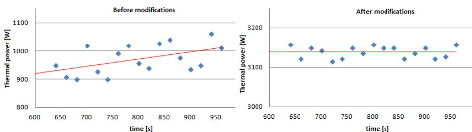
Figure 2. Absorbed thermal power by the water-heated evaporator in function of time
