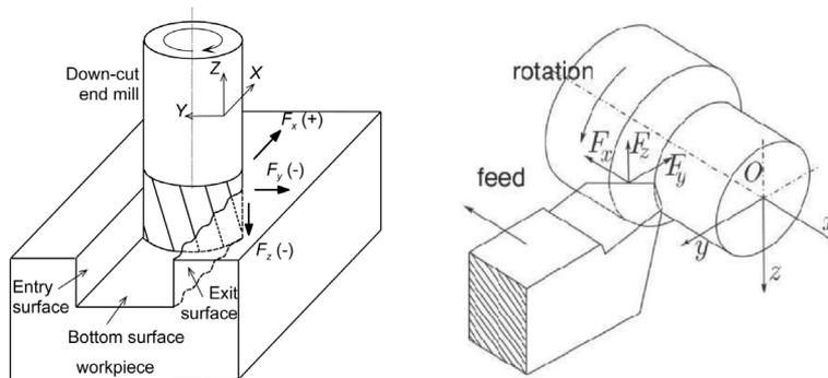
Figure 1. Force components of milling [Luo *et al* 2007] and turning (<http://inspirehep.net/record/1246074/plots>)
