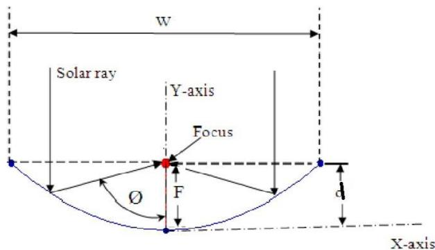
Figure 2. Drawing of Parabolic Trough Solar Collector
