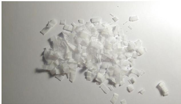
Figure 6. POM C elemental chips
