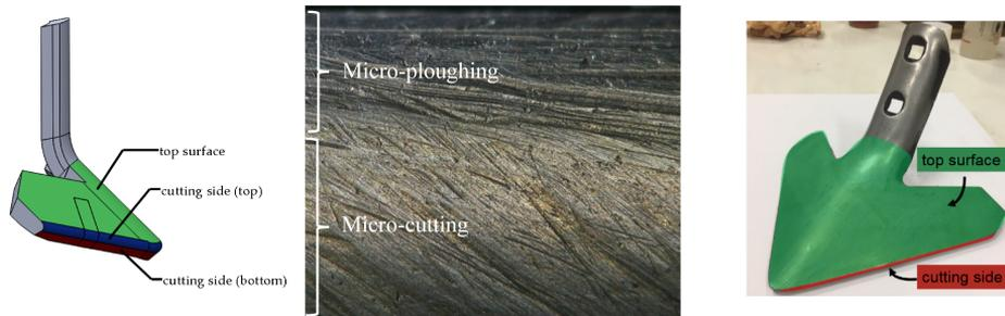
*Figure 6. Segment specific wear mechanism for the agricultural tines used ploughing process*
