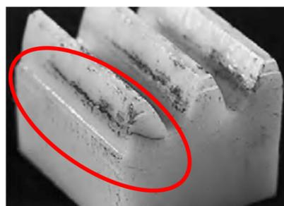
Figure 6. Cracks emanating from the tooth flank close to the pitch diameter [Erhard, 2006]
