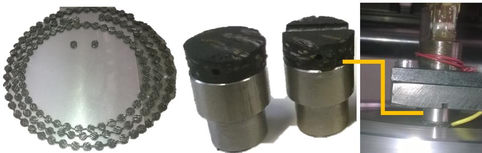
Figure 4. Test specimens cut out from friction facing, additional steel pins for attaching test samples to the system, attached pin
