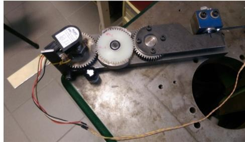
Figure 9. The gear test rig during the measurement
