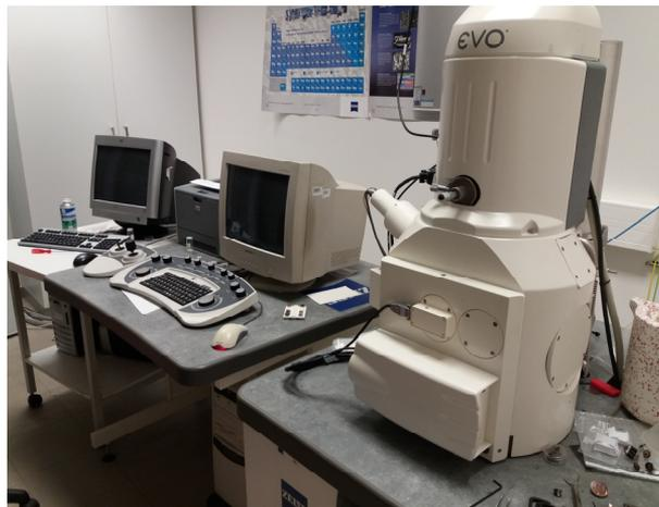
*Figure 3. Scan electron microscopy SEM (Carl Zeiss EVO)*
