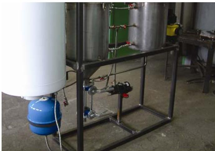
Figure 2. Small scale biodiesel production model
