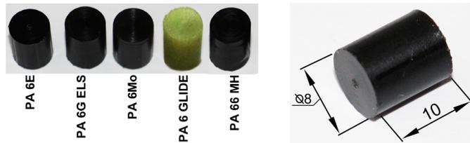
Figure 2. Original forms, colours and dimensions of the tested polymers and composites.
