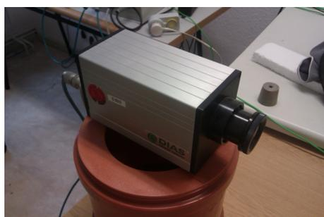
Figure 6. Dias Infrared Camera System Proview 380L
