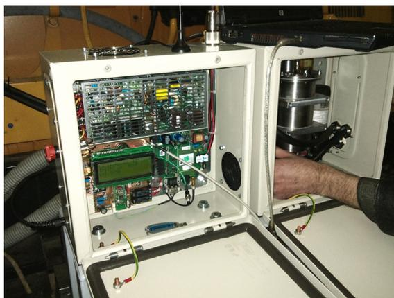
Figure 4. Gas engine oil controlling unit (GOMS)
