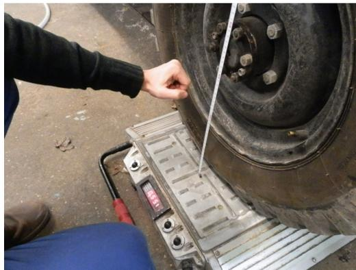
Figure 5. Determining the spring stiffness of the tire
