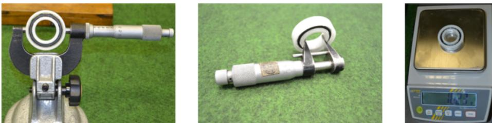
*Figure 6.* Measuring instruments used in the measurement of geometry change
