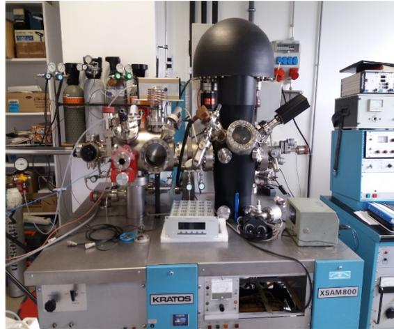
*Figure 2. X-ray photoelectron spectroscopy (XPS)*
