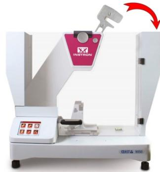
Figure 3. INSTRON CEAST 9050 impact tester
