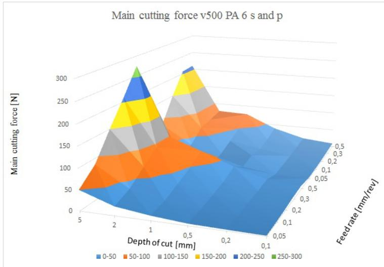
Figure 1. Main cutting forces by using normal surface (front) and polished inserts (behind) (PA 6,  $v = 500$  m/min)
