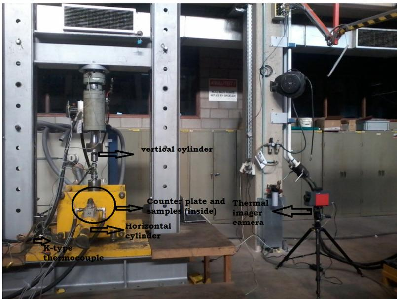
Figure 2. Medium scale experimental setup used for friction and wear measurement located in Laboratory soete, Ghent University, Belgium.
