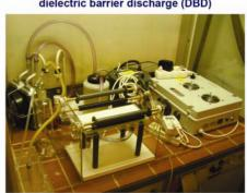
Figure 9. DBD laboratory test equipment used for polymer surfaces. [19]
