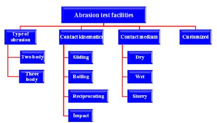
Figure1. Classification of abrasion test facilities.
